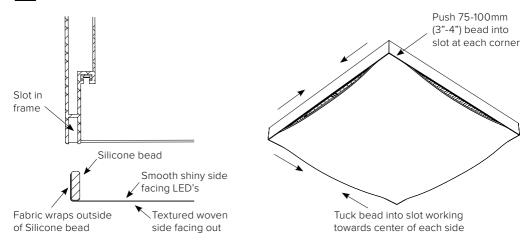
To create luminous ceiling clouds, the FABRICore/FABRICloud luminaires are to be connected together using the clips provided. Alignment of the mounting points prior to installation (5.2) will allow connections to be
